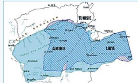
The North Western Sahara Aquifer System (OSS 2008) Geographic distribution of the 'Terminal' Complex' (hatching) and 'Intercalary Continental' (blue) aquifer systems.
